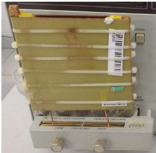
Fig. 3. Sample holder with resin installed in HP 16047C Test Fixture
