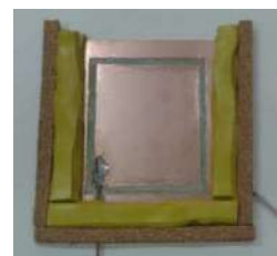
Fig. 2. Tacky tape was used as sealant and cork as spacer
