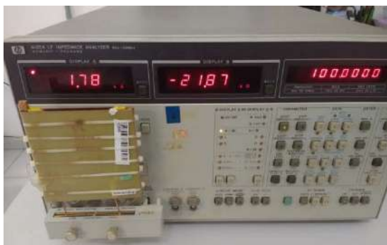
Fig. 4. HP 4192A LF Impedance Analyzer with HP 16047C Test Fixture and sample holder
