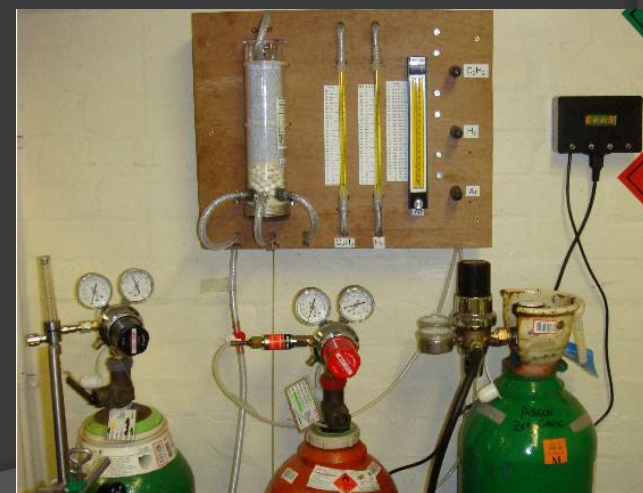
Detail of gas mixture and flow controls
